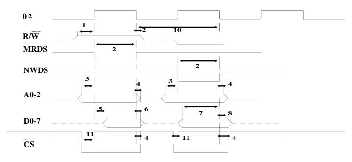
NB On the host side,  $0_2$  is the timing reference and R/W gives the direction of transfer. On the parasite side, the timing and direction are implied by MRDS or NWDS.
