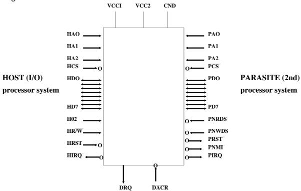
DMA controller on 2nd processor system
